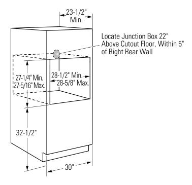
The solid bottom or runners must be level with the bottom of the cutout, or the bottom trim may not install correctly and could interfere with the door opening. If the cabinet does not have a solid bottom, two braces or runners must be installed level with the bottom of the cutout to support the weight of the oven. The runners and braces must support 150 lbs. (68 kg).
